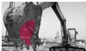
Structures made of Hardox last longer and weigh less, allowing for increased payload. That is why the sign "Hardox In My Body" represents intelligence, performance and economy. Hardox wear steel has unique properties for excavator buckets. Hardox combines extreme hardness and toughness with excellent welding and machining properties. The bucket will last longer, it will keep its original shape and the wear parts will be easy to change.
